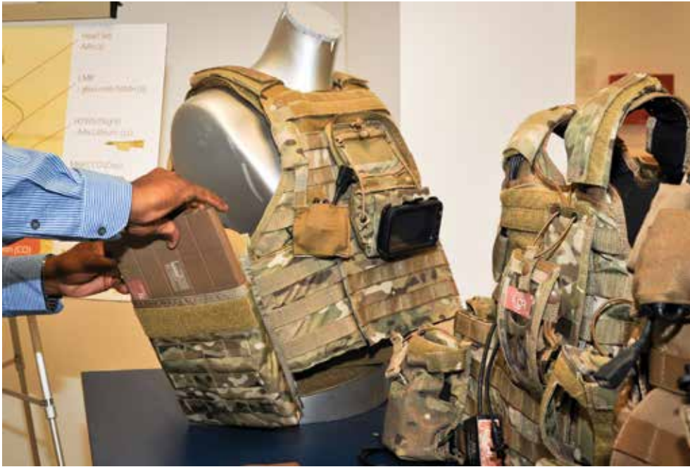
The Conformal Wearable Battery, which is shown being placed into a tactical vest, is flexible and wraps around the body. (Photo: RDECOM)
